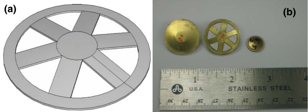
Fig. 2 (a) 3D view of a wagon wheel endcap and (b) photograph showing the cymbal ( left ), wagon wheel ( center ) and standard cymbal ( right ) transducer
